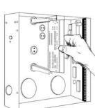
Inside the can, several 2-holed insertion points have been constructed. This allows for either vertical or horizontal placement of the modules. Notice that each insertion point has two sizes of holes – a larger hole and a smaller hole.
